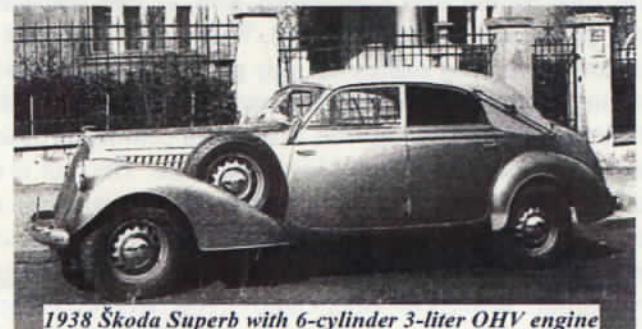
1938 Škoda Superb with 6-cylinder 3-liter OHV engine
